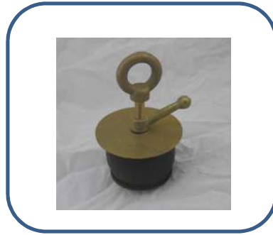
Discription Scupper Plug (Brass) Made from brass and oil resistant rubber. (Stainless or Nylon Scupper Plug are on request) Brass plate thickness: 3mm or 5mm
